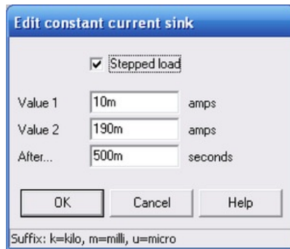
Figure 5.26 Invoking the stepped current feature in PSUD2.
