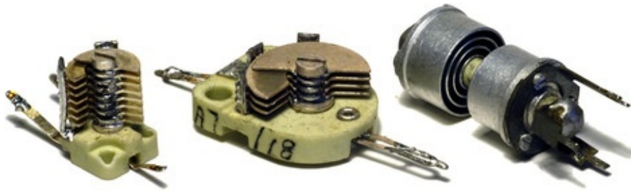
Figure 4.5 Selection of variable air-spaced capacitors. Note that the right-hand trimmer has its vanes disengaged so that they can be seen.
