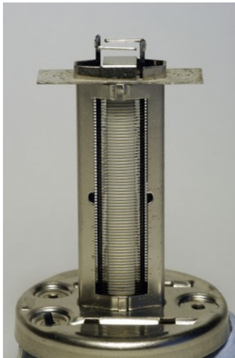
Figure 4.46 Beam-forming plates and cathode/grid structure of QV07-50 VHF dual beam tetrode.
