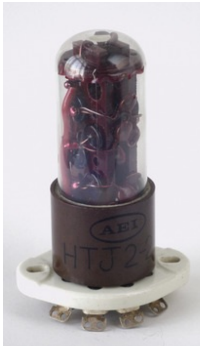
Figure 5.5 Solid-state plug-in replacement for valve rectifier.
