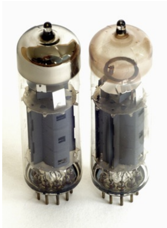
Figure 4.50 The right-hand valve of this pair has almost lost its gettering due to outgassing caused by catastrophic anode overheating.
