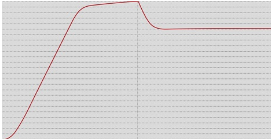
Figure 5.62 PSUD2 simulation shows insufficient voltage and a hint of low frequency undershoot.
