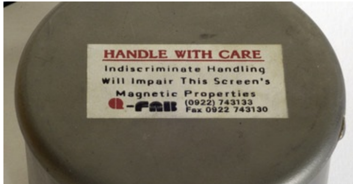
Figure 4.37 The \mu -metal screening can of this transformer demands careful handling.
