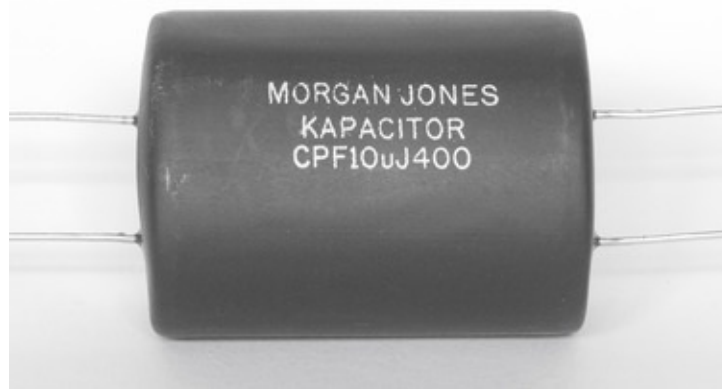
Figure 7.50 Four wire Kelvin connected capacitor.
