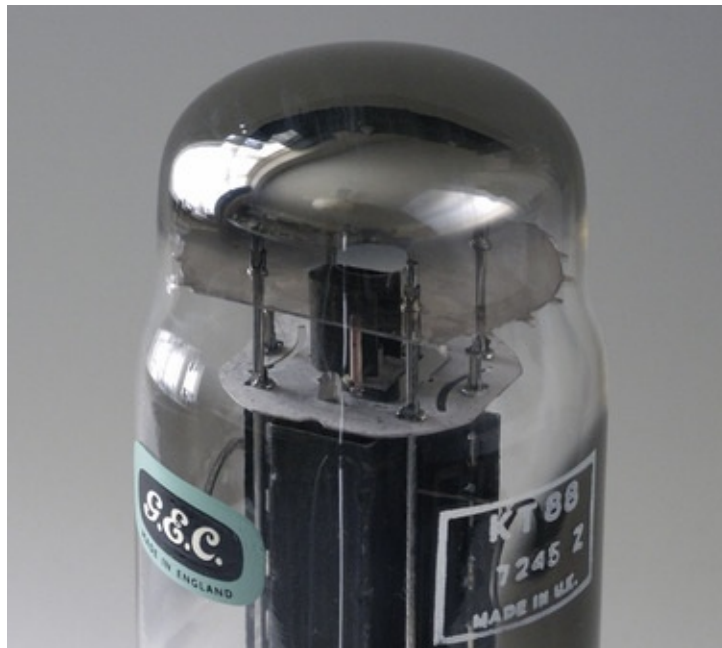
Figure 4.51 View of GEC KT88; note the measures taken to reduce leakage currents.
