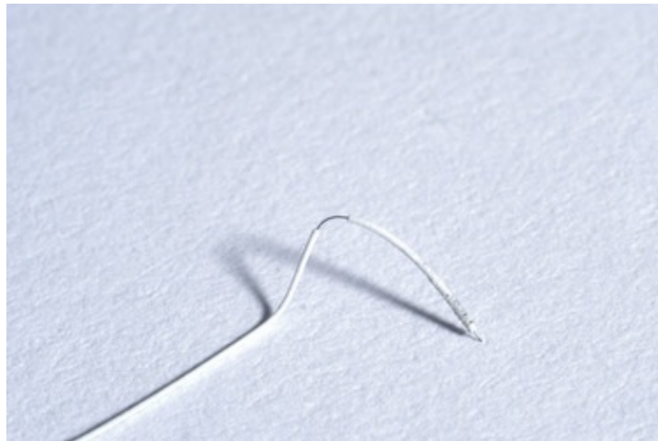
Figure 4.40 6K7 heater filament removed from cathode. The aluminium oxide insulation has been removed at the apex of the hoop to expose the much thinner tungsten filament.
