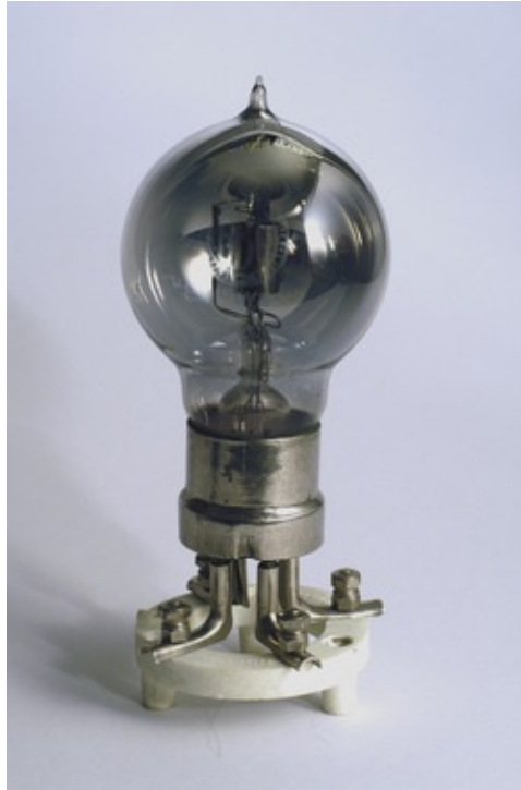
Figure 4.38 R-type valve; note darkening of envelope. (The etched legend declares this valve to be ‘Type approved by Postmaster General BBC’.)
