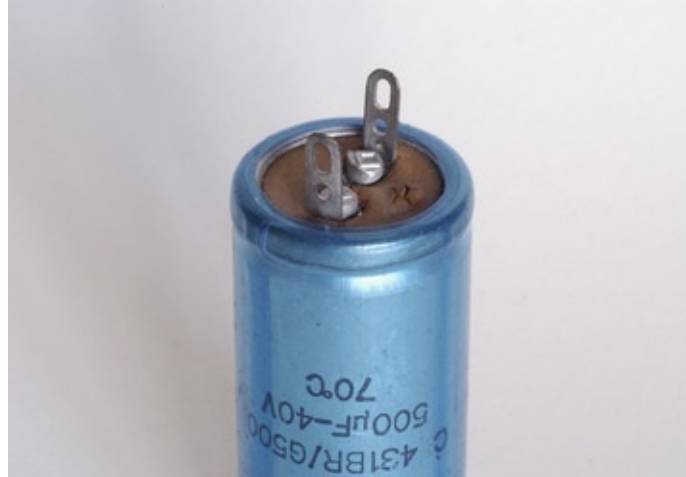
Figure 4.14 Note the bursting pimple that warns of a leaking electrolytic capacitor.
